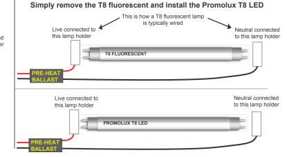
Installing as a Plug-n-Play LED (Type A) Works with pre-heat ballasts only
