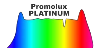
Promolux PLATINUM Balanced Spectrum Small Spikes in Deep Red & Deep Blue Filtered Out Some Small Portions of Visible Spectrum (Yellow) Because they are known to damage fresh food
